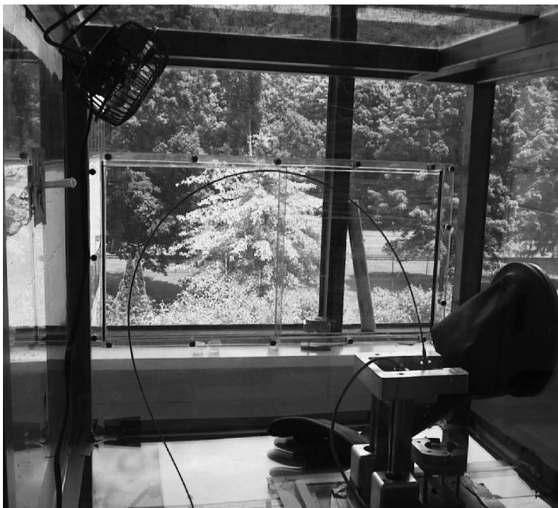
**Figure 4** Aerosol microbial challenge testing chamber unit
