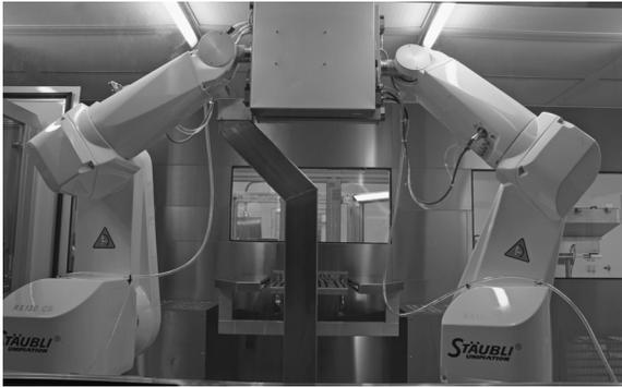
**Figure 1** Illustration of the clean room class 100/Grade A/ISO 5 used for vial body and stopper molding, followed by robot assembly.
