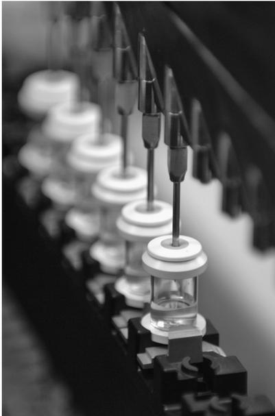
**Figure 2** Piercing of the vial showing the tight contact between stopper and needle.
