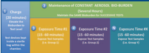
Figure 8: Proposed steps in an aerosol microbiological challenge test. Step-P: pre-test activities. Step 1: charge, to elevate the chamber bioburden to test levels using the programmable nebulizers. Step 2: maintenance of bioburden using the programmable nebulizers for successive tests. Step 3, Step 4, and Step N: exposure time during the maintenance (Step 2) for test units or test groups; the exposure time of 15 to 60 minutes is suggested considering the settling rates calculated below (see Table VI).
